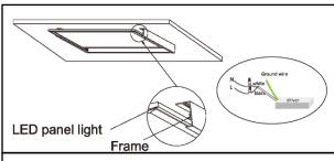
5. Connect the input ends of the driver to those of N/L wire. Make sure the connection is tightly fastened and the power is off before connecting in case of electric shock.
