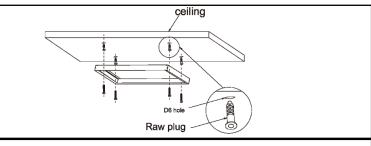
2.Drill four D6mm holes on the ceiling, install the raw plug and fix the frame on the ceiling.
